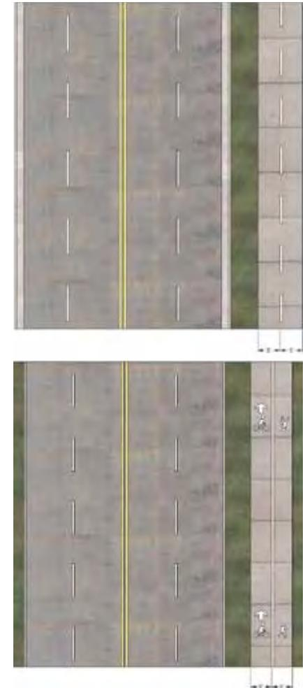
**Sidepath sections.** Sidepath width and construction standards are similar to those for multi-use trails. Top: Two-way sidepath along an arterial, a typical accommodation on contemporary streets. Above: One-way cycle track concept separates pedestrian from bicycle traffic. Bicycles move in the direction of traffic.
