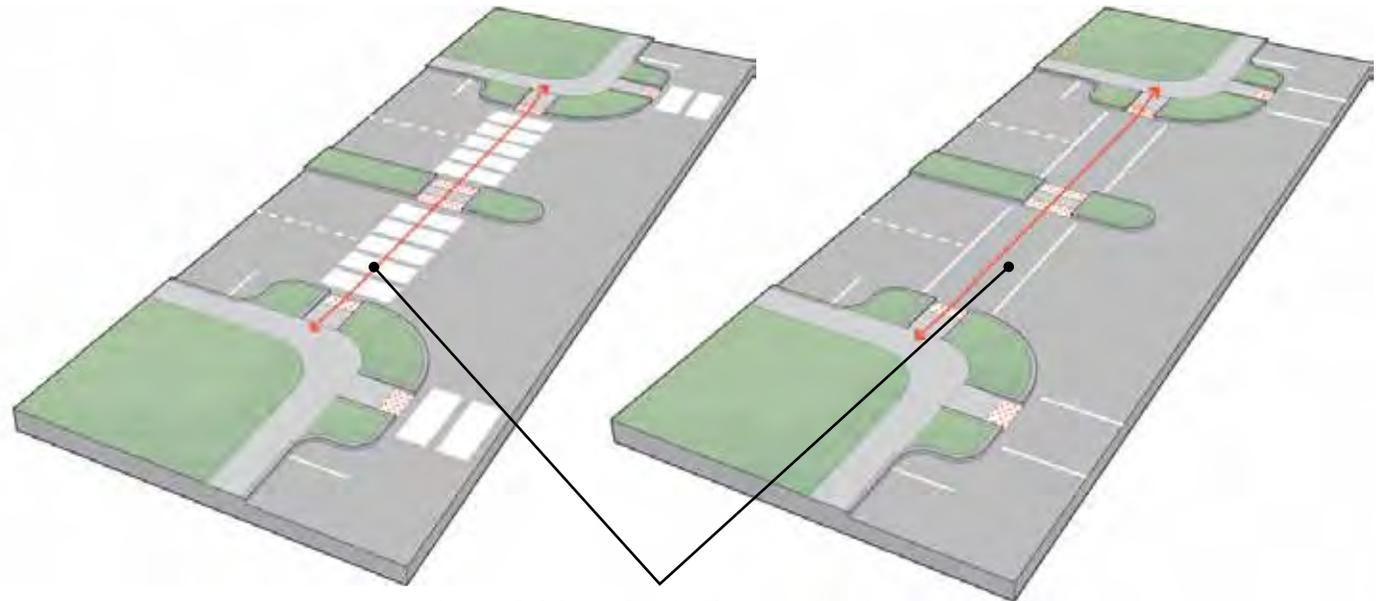
**Ladder Striping vs Parallel Lines.** Ladder striping can be seen better by motorists and pedestrians, while parallel lines is a more affordable application.
