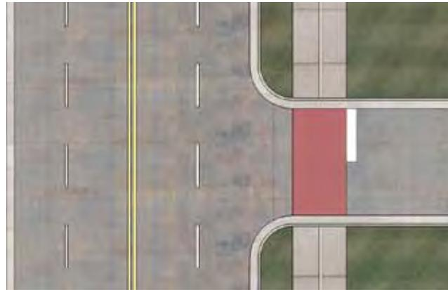
**Crossing Definition.** Sidepath/cycle track crossings should be defined for maximum visibility. Colored or textured surfaces can be effective in these situations. A clear stop bar should also be used with advisory signage, to discourage motorists from blocking the track.
