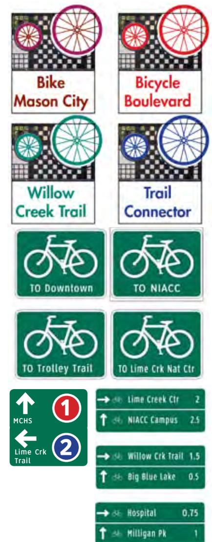
Above: Possible system components for Mason City. From top: Identification signs, destination signs, route intersection, and mileage blade signs.
