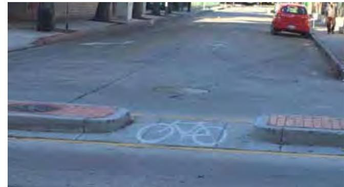
**Arterial street crossings for bicycle boulevards and pedestrian corridors.** From left: Crossing median concept for urban corridor by RDG.; Median installation in Las Vegas; diverter island in Los Angeles.
