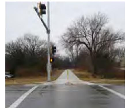
**Hybrid Beacon.** The hybrid beacon (or HAWK signal) functions somewhat like school bus warning signals. It is dark when not in use. When actuated by a pedestrian, a flashing and then solid yellow light warns motorists to slow; a solid red light paired with a walk signal stops traffic and gives the right-of-way to the pedestrian. Users report a high degree of motorist compliance and a positive effect on pedestrian safety.
